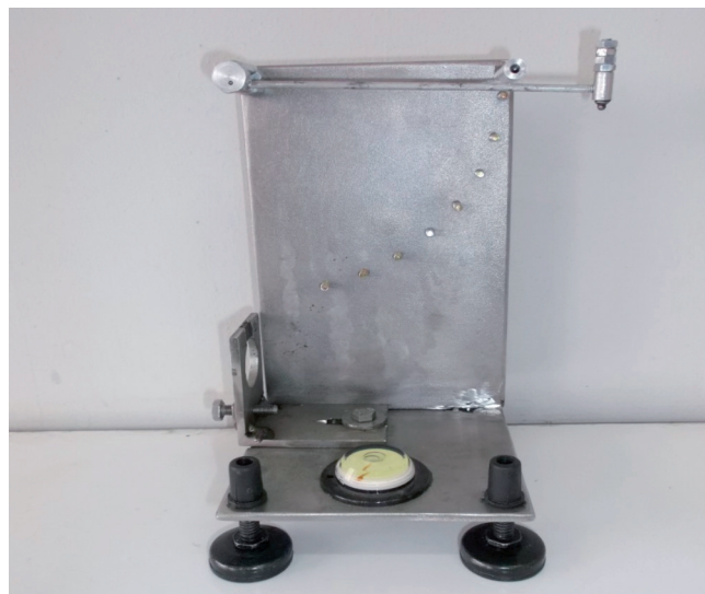
Figure 1. Mechanical device used to induce pitting. Impact levels 0.00342 and 0.0107 J were calculated as the impact energies on the fruit when the pendulum moved from an angle of 45° and 90° respectively with regard to the vertical position of the pendulum.
