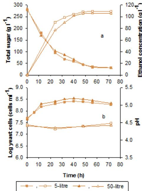
**Fig. 6** Fermentation kinetics during batch ethanol production from the sweet sorghum juice supplemented with 8 g l<sup>-1</sup> of DSY in 5-litre and 50-litre bioreactors. (a) total sugar (closed symbol) and ethanol concentration (open symbol), (b) log viable yeast cells (closed symbol) and pH (open symbol).
