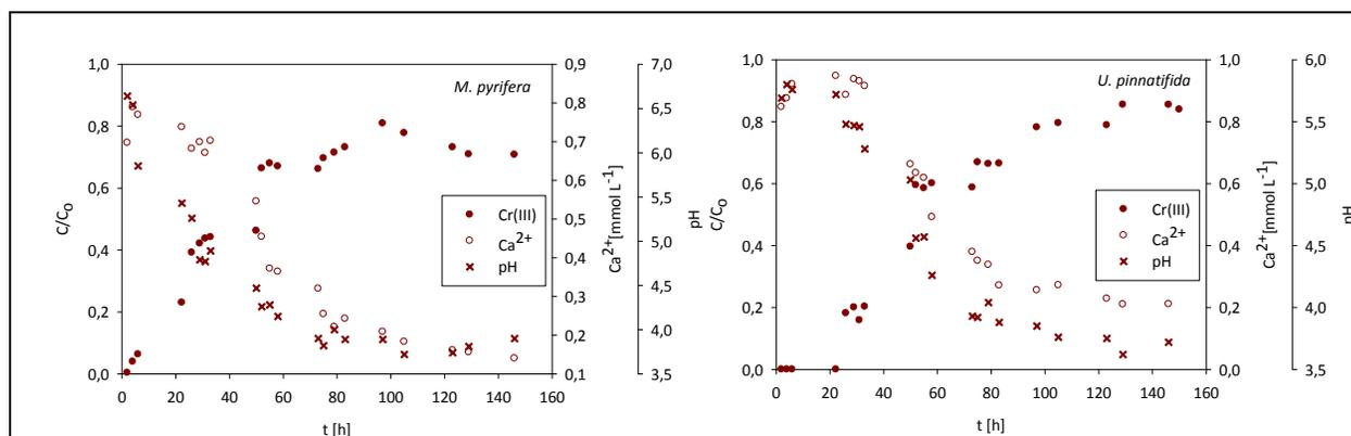
**Fig. 2** Cr(III) breakthrough curves for calcium-treated *M. pyrifera* and *U. pinnatifida* biomasses. Empty and closed circle symbols represent calcium release and Cr(III) concentration in the eluate, respectively, while cross symbols indicate pH behaviour during Cr(III) uptake.
