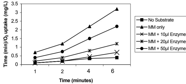
Fig 1: Influence of varying methylmercaptan (MM) oxidase titres on degradation of MM at pH 8.0
