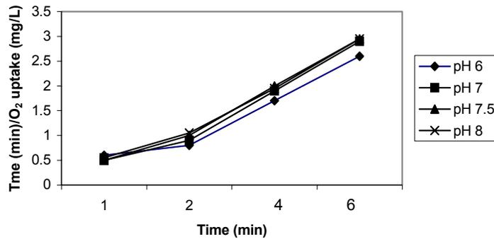
Fig 3: Influence of pH on methylmercaptan oxidase using phosphate buffer
