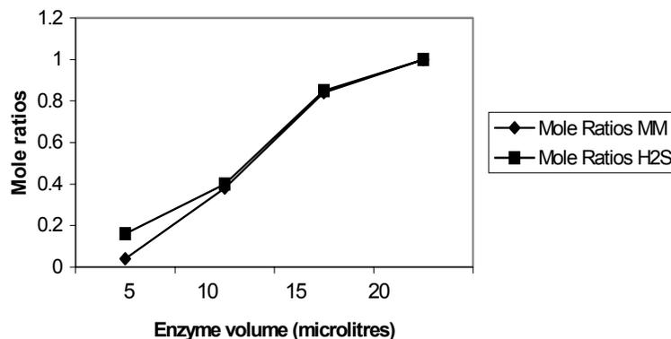
**Fig 5:** Influence of methylmercaptan (MM) oxidase volume on degradation of methylmercaptan
