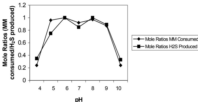
**Fig 4:** Comparison of methylmercaptan (MM) consumption and H<sub>2</sub>S production at varying pH levels
