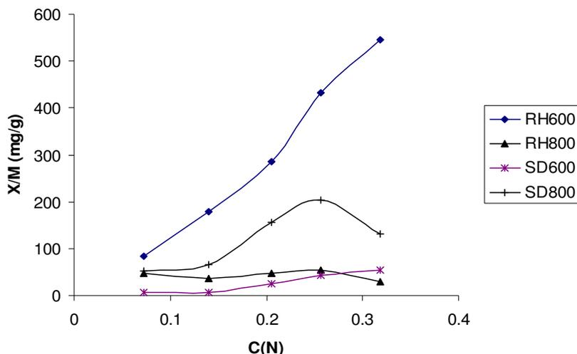
Fig.1: Acetic acid adsorbance isotherm on activated carbon
