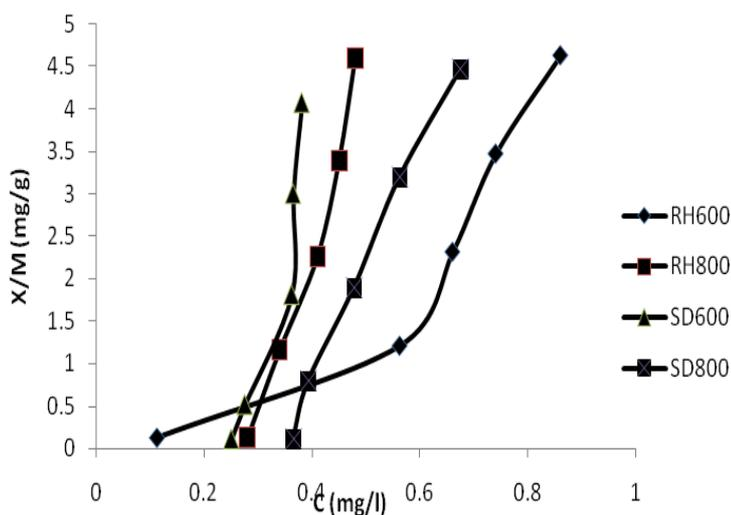
Figure 4: Adsorbance of cadmium (II) ion from aqueous solution
