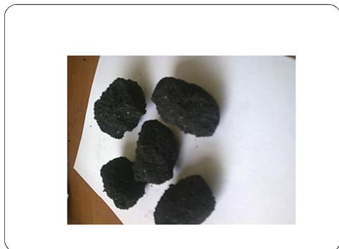
Fig 1: Hand- molded briquettes
