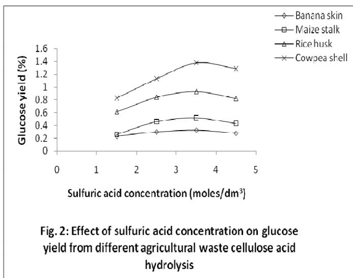
Fig. 2: Effect of sulfuric acid concentration on glucose yield from different agricultural waste cellulose acid hydrolysis
