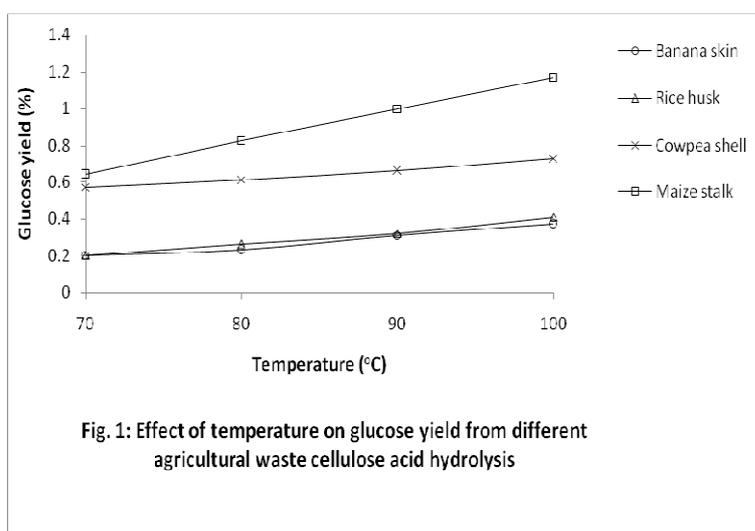
Fig. 1: Effect of temperature on glucose yield from different agricultural waste cellulose acid hydrolysis
