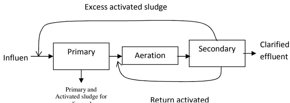
**Fig. 1:** The flow of materials through an activated sludge employed in the sewage treatment system.
