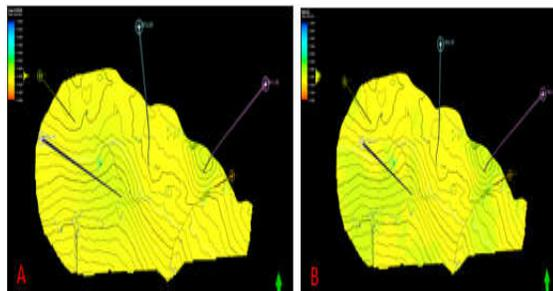
**Fig 14** (A) and (B) Showing the water saturation distribution across J10 reservoir in deterministic and stochastic probability conditions respectively
