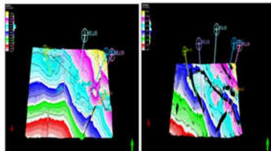
Fig 7: (A) and (B) showing the Depth maps generated for Horizons J10 and J3 respectively.
