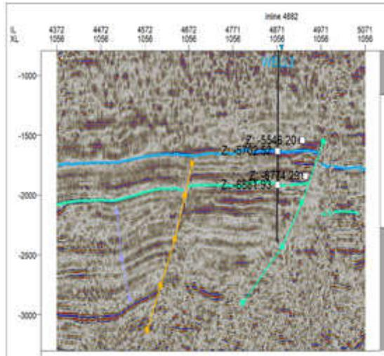
Fig 5: Showing 2 horizons picked and faults interpreted
