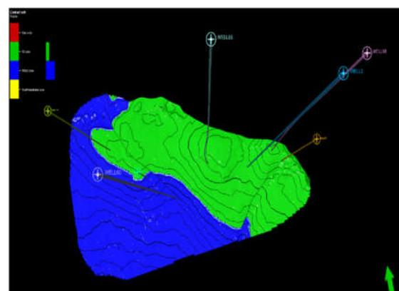
Fig 20 showing the Oil-Water contact model for reservoir J3.
