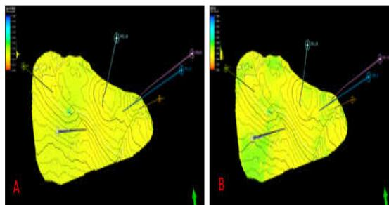
**Fig 15** (A) and (B) Showing the water saturation distribution across J3 reservoir in deterministic and stochastic probability conditions respectively
