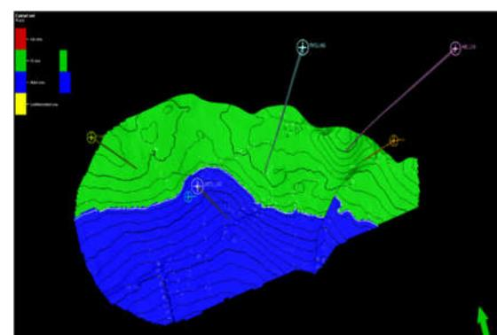
Fig 19 showing the Oil-Water contact model for reservoir J10
