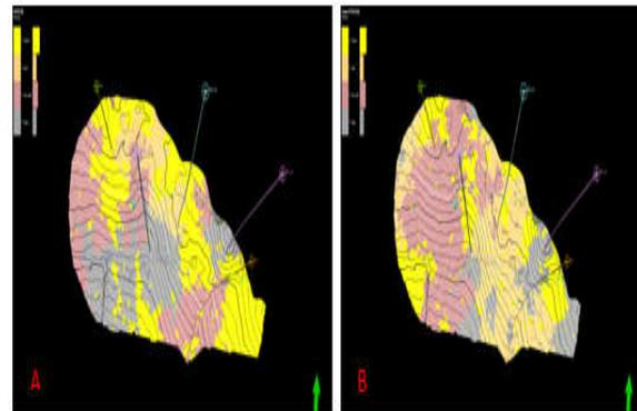
Fig 8 (A) and (B) Showing the Facie Models for horizon J10 in stochastic and deterministic probability conditions respectively
