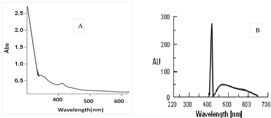
**Figure 1:** UV-visible absorption (A) and fluorescence spectrum (B) spectrum of the silver nanoparticles
