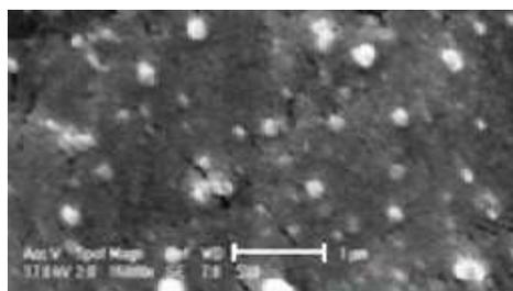
**Figure 3:** SEM image of the silver nanoparticles
