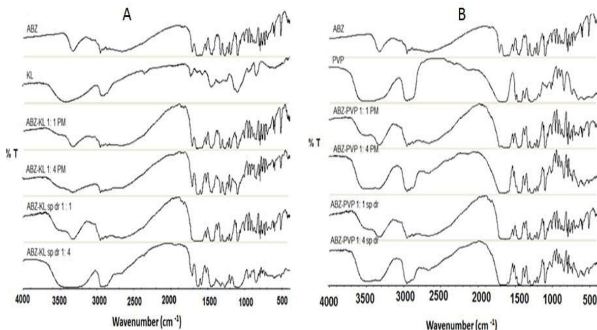
**Fig 3:** A = FTIR spectra of ABZ-KL spray dried and physical mixtures in drug: polymer ratios 1: 1 and 1: 4 compared to the individual components, and B = FTIR spectra of ABZ-PVP spray dried and physical mixtures in drug: polymer ratios 1: 1 and 1: 4 compared to the individual components
