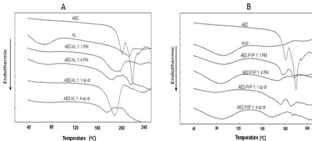
**Fig 2:** **A** = DSC thermograms of ABZ-KL spray dried and physical mixtures in drug: polymer ratios 1: 1 and 1: 4 compared to the individual components, and **B** = DSC thermograms of ABZ-PVP spray dried and physical mixtures in drug: polymer ratios 1: 1 and 1: 4 compared to the individual components
