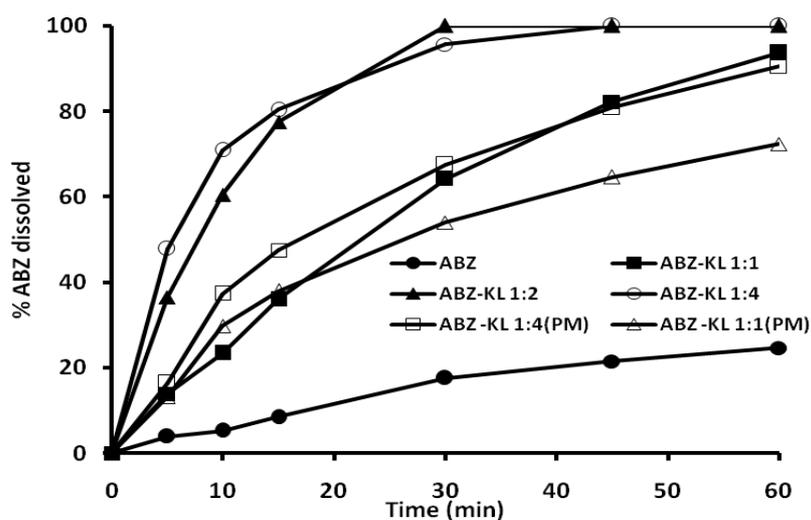
**Fig 4:** Dissolution profiles of ABZ-KL spray-dried systems compared to the corresponding physical mixtures (PM)
