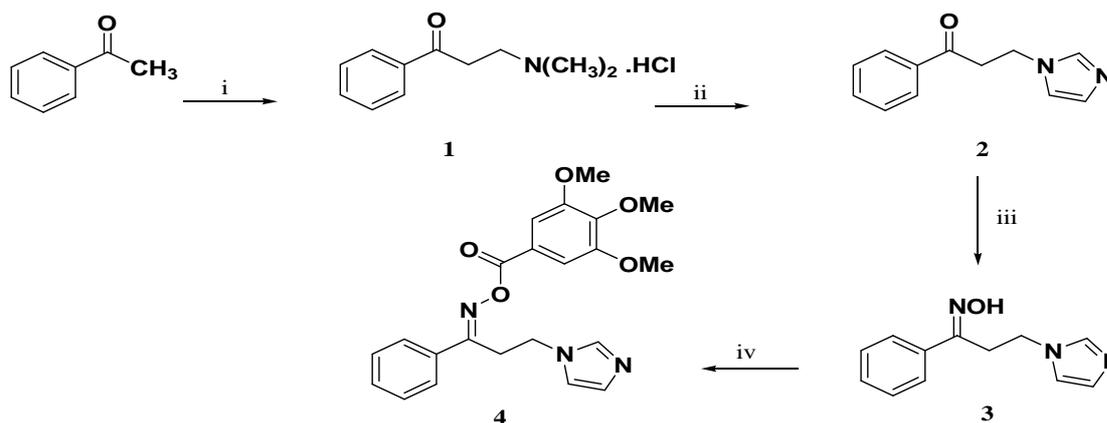
**Scheme 1:** Synthesis of the title compound **4**. Reagents and conditions: i) HN(CH<sub>3</sub>)<sub>2</sub>.HCl, (CH<sub>2</sub>O)<sub>n</sub>, conc. HCl, ethanol, reflux, 2 h; ii) Imidazole, water, reflux, 5 h; iii) H<sub>2</sub>NOH.HCl, KOH, ethanol, reflux, 18 h; iv) 3,4,5-Trimethoxybenzoic acid, EDCI.HCl, DMAP, DCM, rt, 18 h.
