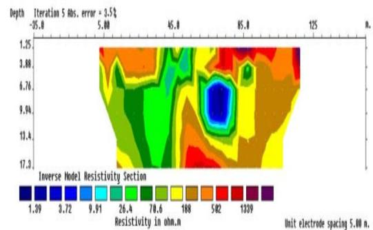
**Fig. 4.1(d)** 2D electrical resistivity imaging sections along profile 4
