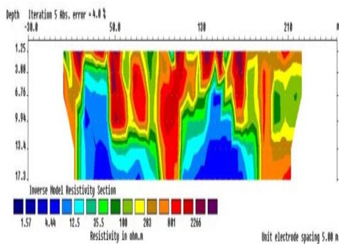
**Fig. 4.1(a)** 2D electrical resistivity imaging sections along profile 1
