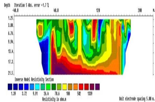
**Fig. 4.1(c)** 2D electrical resistivity imaging sections along profile
