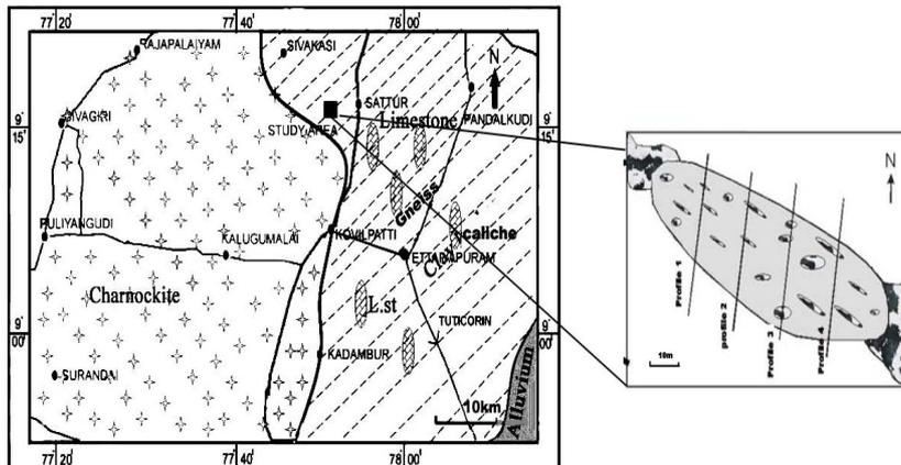
**Fig.1** Geological map of the surveyed area (left). 2D electrical resistivity imaging conducted along profiles 1-4 (right).
