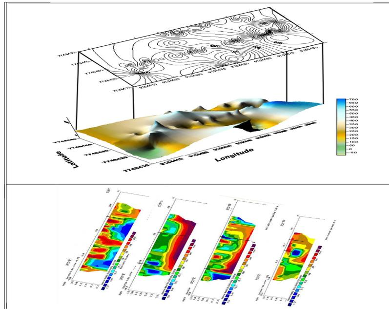
**Fig.5.** Shows the 3D model of 2D electrical resistivity imaging pseudosection along the profile in the banded iron ore deposits at Elayiram Pannai, Sattur Taluk, Virudhunagar District, Tamilnadu
