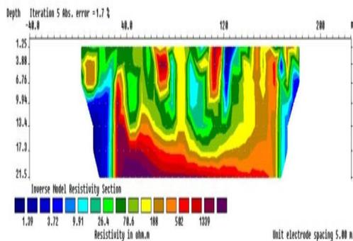
**Fig. 4.1(b)** 2D electrical resistivity imaging sections along profile 2
