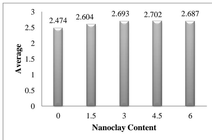
Fig 2. Soil compressive strength with different percents of nanoclay
