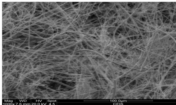
**Fig 3.** SEM image of quartz filter paper showing collected air-borne dust
