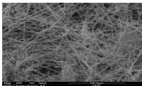
**Fig 2.** SEM image of quartz filter paper before sample collection
