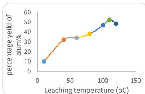
**Fig 5:** Effect of leaching temperature on the extraction of the alum (leaching time: 1.5 h; acid concentration: 4M; particle size: 100 µm,)
