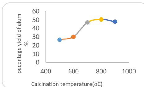
Fig 2: Effect of calcination temperature on the extraction of alum (time: 1.5 h, particle size:  $100\text{ }\mu\text{m}$ )
