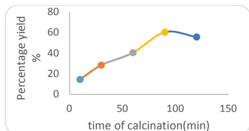
**Fig 3:** Effect of calcinations time on the extraction of alum (particle size: 100 µm, temperature: 800°C).
