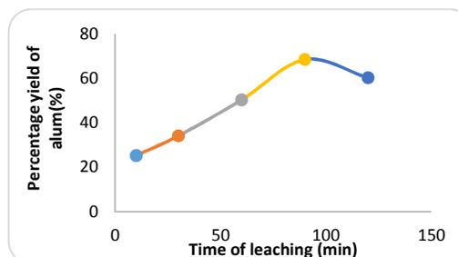
**Fig 6:** Effect of leaching time on the extraction of alum (acid concentration: 5M; particle size: 100 µm; temperature: 110°C)
