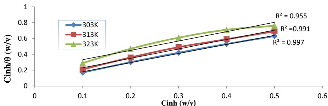
Fig 7:Langmuir adsorption isotherm of CSAE on mild steel in 0.5M HCl solution at different temperatures
