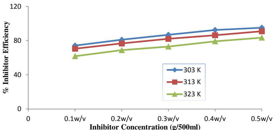
**Fig 3** Average Percentage Inhibition Efficiency (%IE) of different concentrations of CSME for the Inhibition of Mild Steel corrosion in 0.5 M HCl solution at different temperatures
