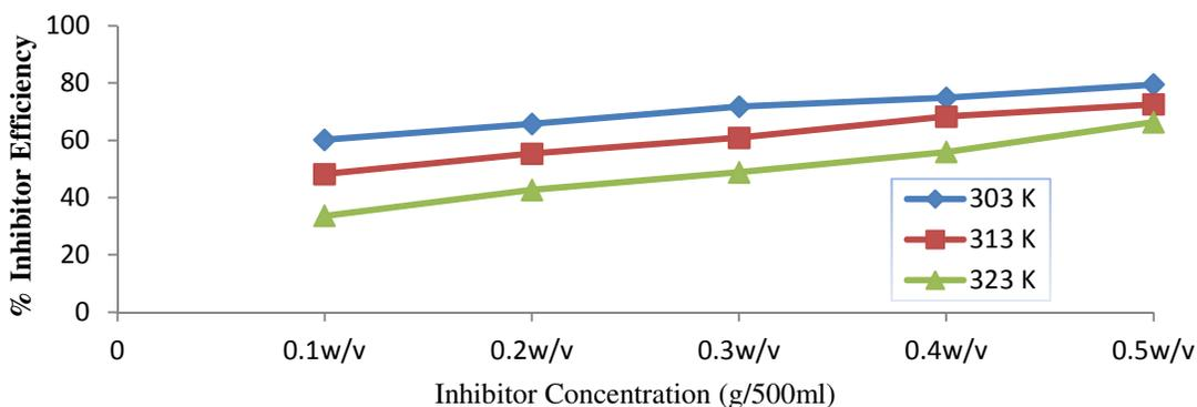
**Fig 4** The Average Percentage Inhibition Efficiency (%IE) of different concentrations of CSAE for the Inhibition of Mild Steel corrosion in 0.5M HCl solution at different temperatures
