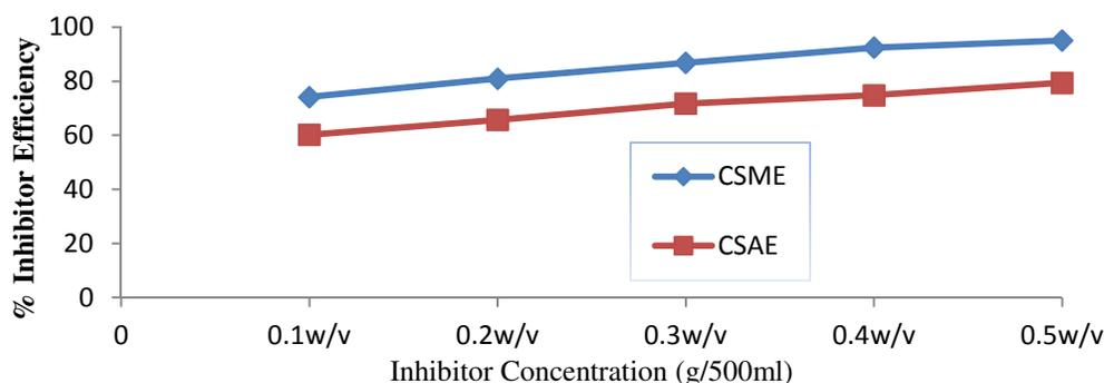
**Fig 5:**The Average Percentage Inhibition Efficiency (%IE) of CSME and CSAE for the Inhibition of Mild Steel corrosion in 0.5M HCl solution at 303K.
