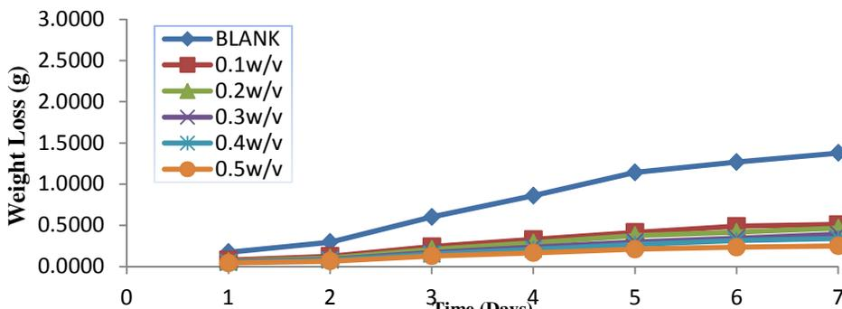
Fig 2 Variation of Weight Loss with Time for Mild Steel Coupons in 0.5 M HCl solution containing different concentrations of CSAE at 303 K
