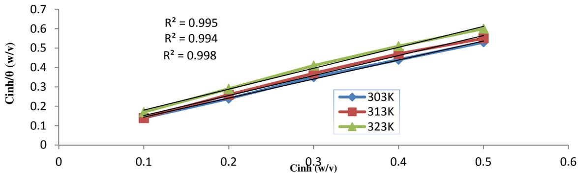
Fig 6 Langmuir Adsorption Isotherm of CSME on Mild Steel in 0.5M HCl solution at different temperatures
