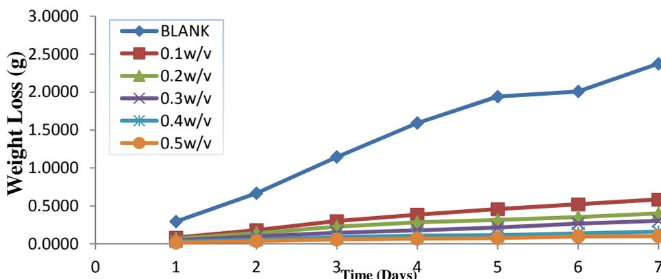
Fig 1 Variation of Weight Loss with Time for Mild Steel Coupons in 0.5 M HCl solution containing different concentrations of CSME at 303 K
