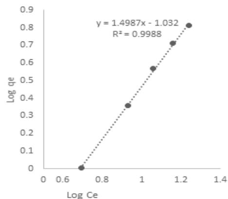
Fig 7: Freundlich Isotherm plot for naphthalene adsorption on snail shell
