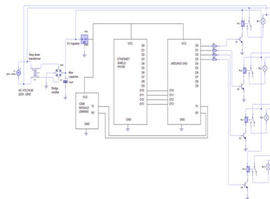
Fig 3: Circuit diagram of the smart switch
