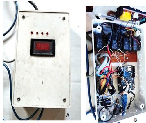
Fig 5: Smart switch prototypes: (A) Enclosed, (B) Opened to reveal components
