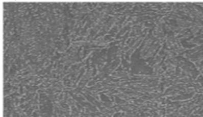
**Plate 2:** Distribution of tempered microstructure of 0.25-0.35% C grade of medium carbon steel quenched from 800 °C. (500x).
