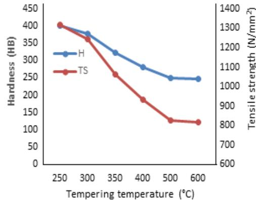
Fig 4: Hardness and Tensile strength at varying tempering temperatures (previously normalized and quenched at 850 °C)
