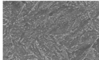
**Plate 4:** Distribution of tempered microstructure of 0.25-0.35% C grade of medium carbon steel quenched from 900 °C (500 ×)
