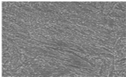
**Plate 1:** Distribution of tempered microstructure of 0.25-0.35% C grade medium carbon steel quenched from 750 °C (500 ×)
