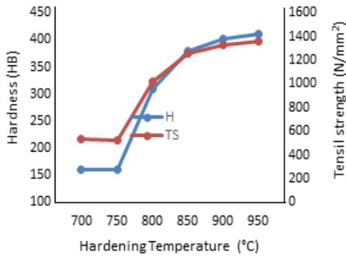
Fig 2: Hardness and Tensile strength at various hardening temperatures after normalizing at 850°C
