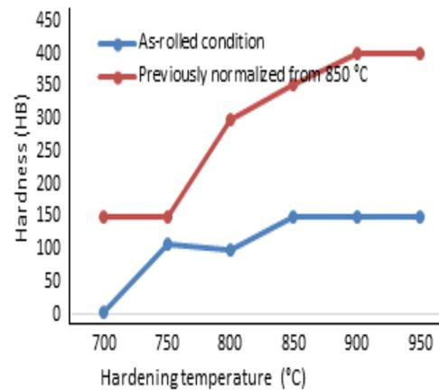
Fig 5: Hardness of the steel in the as-rolled condition and after normalization
