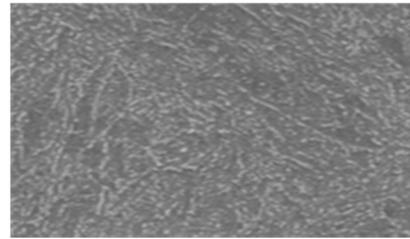
**Plate 3:** Distribution of tempered microstructure of 0.25-0.35% C grade of medium carbon steel quenched from 850 °C (500 ×)
