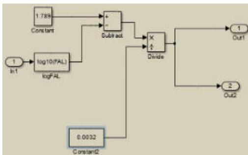
**Fig 2:** Simulink Subsystem for Calculating the Degree of Polymerisation, DP
