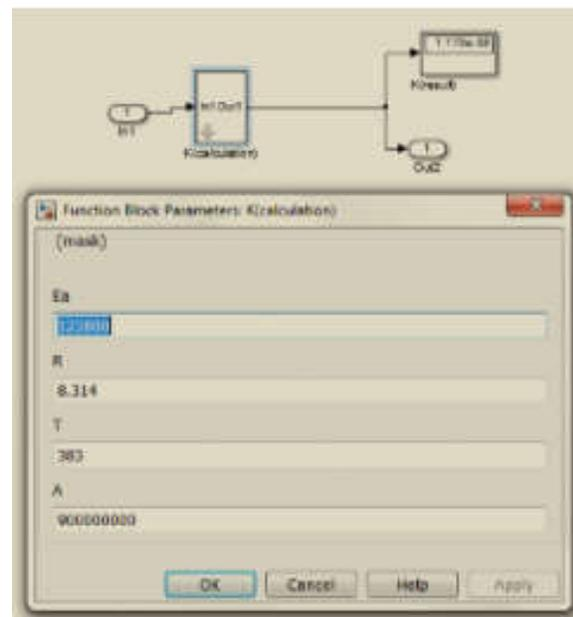
**Fig 4:** Simulink Model Interphase for Calculating the Ageing Rate Constant,  $k$
