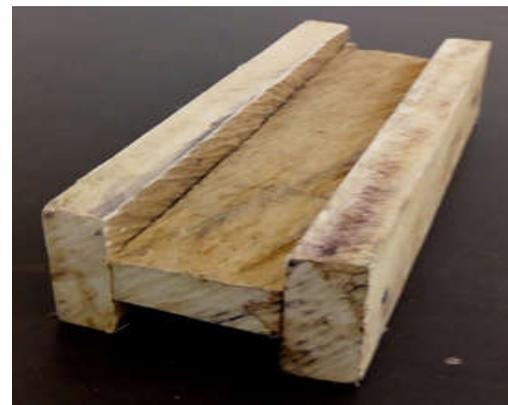
Plate 1 Showing I-Section Test Specimen
