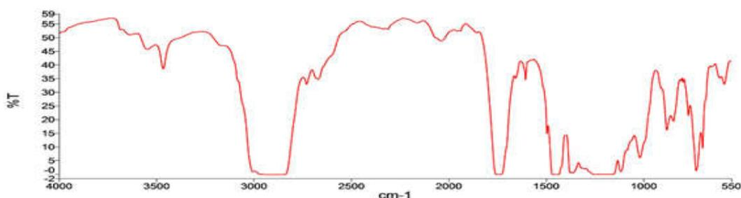
**Fig. 6:** FT-IR spectrum of produced biodiesel from *A. cunninghamiana* seed oil
