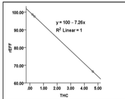
**Fig 9:** Regression model establishing the significant relationship between total hydrocarbon content (THC) (independent var.) and remediation efficiency (rEFF) (dependent var.) during the study
