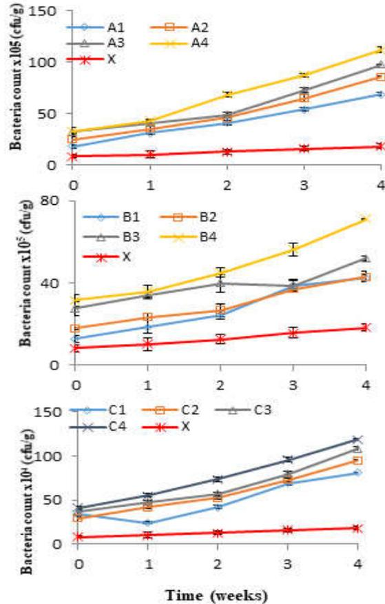
**Fig 3:** Hydrocarbon utilizing bacteria count (HUBC) of crude oil contaminated soil treated with various amendments
