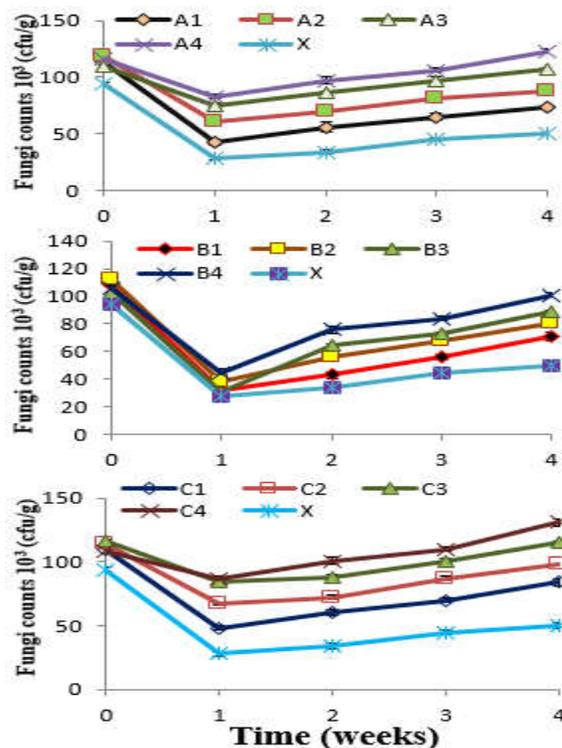
Fig 2: Total heterotrophic fungi count for crude oil contaminated soil treated with various amendments.
