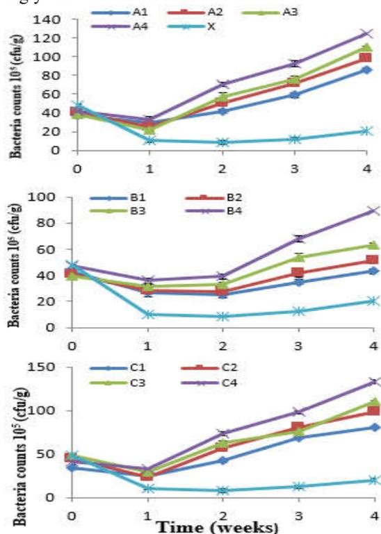
Fig 1: Total heterotrophic bacteria count for crude oil contaminated soil treated with various amendments
