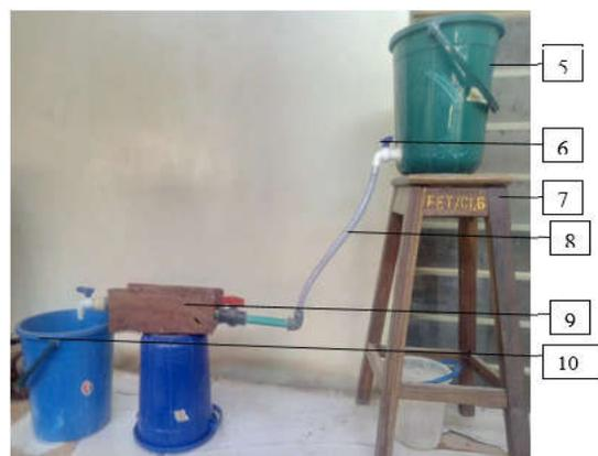
Fig 2. Magnetic treatment unit for the wastewater: Legend: 5 = Storage tank, 6 = control tap, 7 = stool, 8 = hose, 9 = magnetic field unit, 10 = collector for the wastewater
