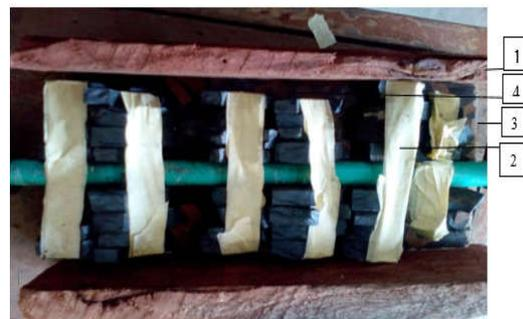
**Fig 1.** Arrangement of permanent magnet on the PVC pipe for the wastewater treatment: Legend: 1 = wooden housing, 2 = paper tape, 3 = 0.5inch PVC pipe, 4 = permanent magnet
