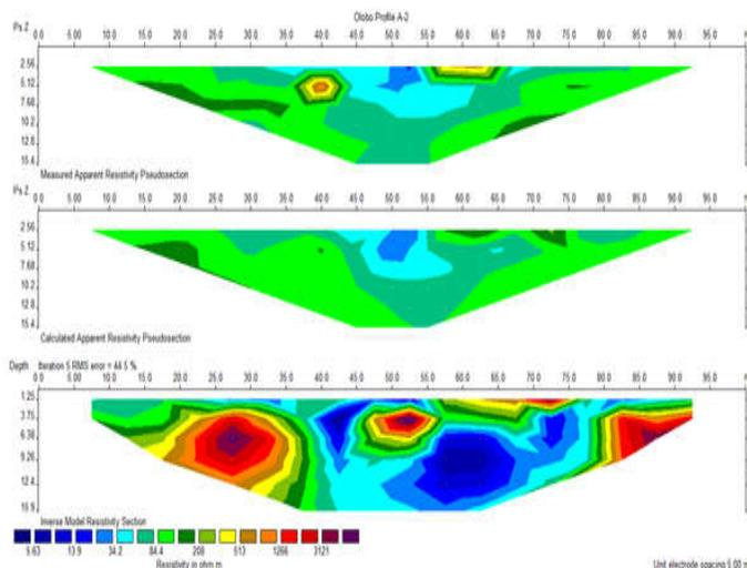
Fig 3. Inverse resistivity model section of profile 2. The section is the result of the simultaneously processed horizontal profiling and vertical profiling
