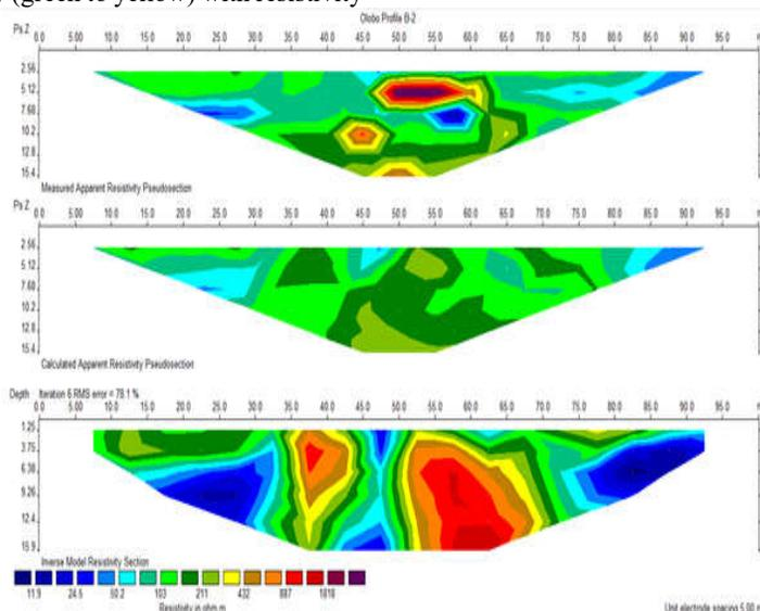
Fig 2. Inverse model resistivity section of profile 1. The model is the result of the simultaneously processed horizontal profiling and vertical profiling data.
